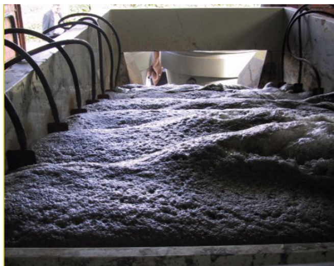
Illustration of an electro coagulation unit in a pig farm at Errentería (Spain). Photo: Lekuona (2004)
