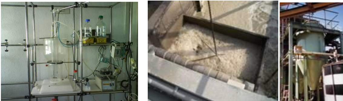
Laboratory reactor for struvite precipitation at GIRO (Spain), left, and two views of a struvite producing plant from animal slurry, courtesy of Dr. Kazuyoshi Suzuki (Japan)
