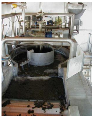
Mixing chamber of pig manure with a polymer followed by a rotating screen at Pigneto di Prignano, MO, Italy, (left) courtesy of SELCO MC; (a) coagulation, (b) patch flocculation, schematic (Hjorth et al. , 2008) (right).
