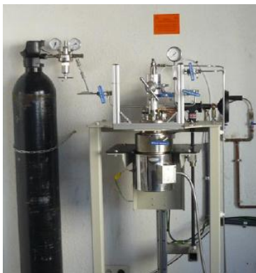
Lab equipment for T/P treatment (left) at GIRO (Spain) and integrated pasteurization unit (right) post-anaerobic digestion at Lemvig (Denmark)
