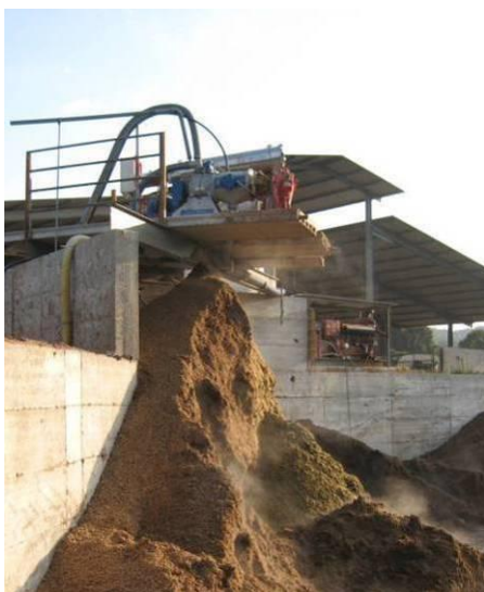
Illustration of a screw press (left) at Balenyà (Spain), and a scheme of an screw press system (right) from Burton (2007).
