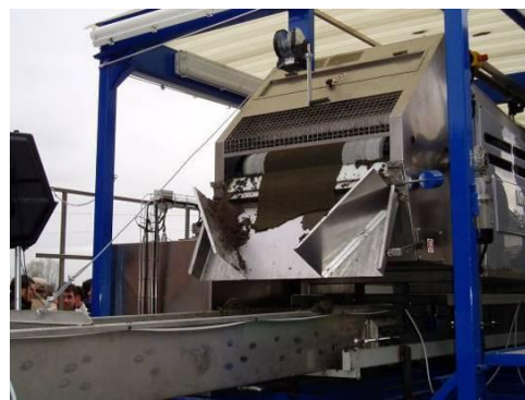
Illustration of a rotary press at Tyndall Farm (SC, USA) (left), and a filter belt applied to pig slurry courtesy of Mr. Martínez-Almela (right).
