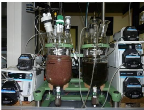
Illustration of lab-scale reactors using totally autotrophic N-removal combining partial nitrification and anammox, at the Laboratory of Coastal Plains Soil, Water and Plant Research Centre. ARS-USDA. Florence (SC-USA).
