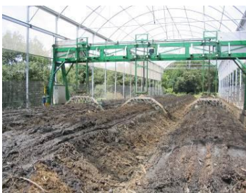
Illustration of pig farm-scale bio drying: at Les Garrigues county (upper row) and at Torelló (lower row), Catalonia, Spain. These examples are pilot experiences.
