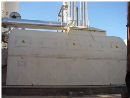
Illustration of a dryer (left) and image of the dried product (right) at the TRACJUSA pig manure treatment plant (Juneda, Spain).
