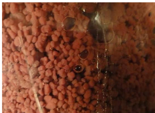
Illustration of lab-scale reactors using totally autotrophic N-removal combining partial nitrification and anammox, at the Laboratory of Coastal Plains Soil, Water and Plant Research Centre. ARS-USDA. Florence (SC-USA).
