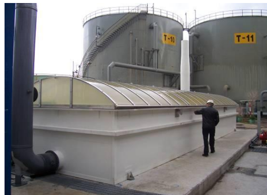
Illustration of the biofiltration unit at TRACJUSA (Juneda, Spain), left, and DMT Environmental Technology (The Netherlands) www.dmt-et.nl , right
