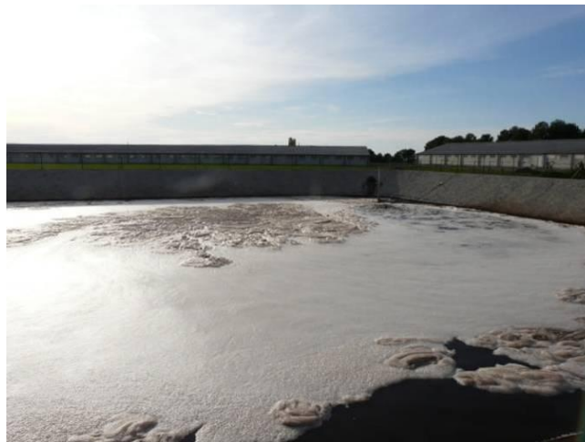
Illustration of an aerobic digestion system based on intermittent aeration aiming to N-removal in a pig farm at Almacelles (Spain).
